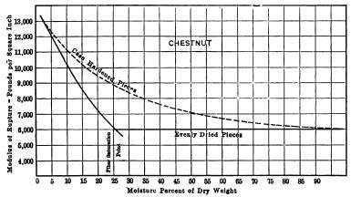
Fig. 15.—Effect of casehardening upon the form of the moisture-strength curve in bending tests. The upper curve is from casehardened specimens, the lower curve from uniformly dried specimens.
